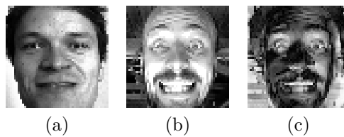
Figure 5.5: (a) Owner reference sample of the database (b) Not-owner observation sample (c) Difference image, labeled negative.
