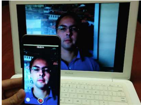
Figure 2.3: Demonstration of a video replay attack where an image sequence is collected via smartphone from a notebook screen (the spoof medium) from a video found online [54].
