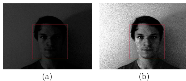
Figure 5.3: (a) Image before histogram equalization. (b) Image after histogram equalization.
