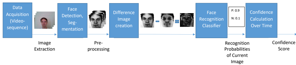
Figure 7.5: Overview of modules used in the continuous mobile face authentication system.
