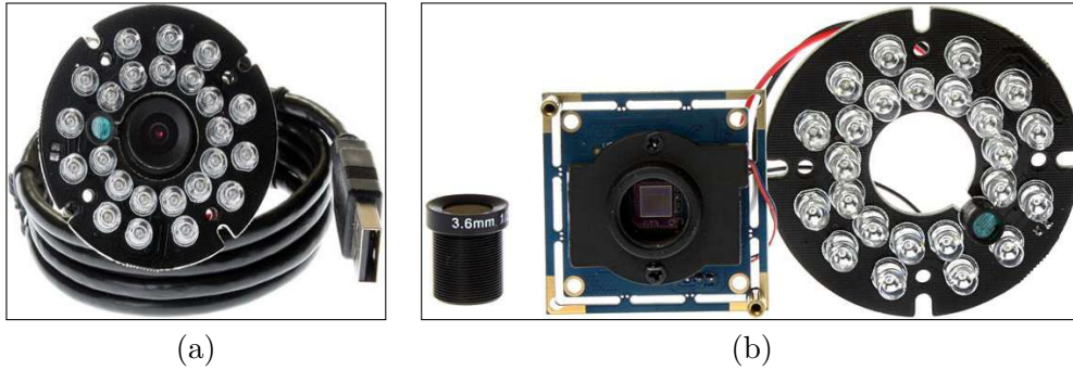
Figure 6.5: CCD camera [73]: (a) camera block, and (b) disassembled camera.
